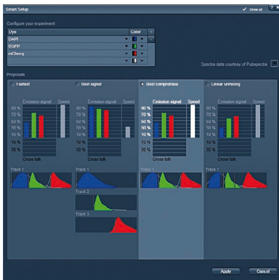
Smart setup allows automatic setting of imaging parameters depending on your preferences for acquisition speed and signal quality.
