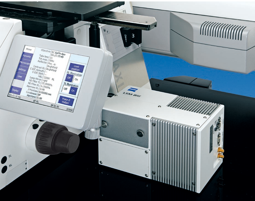
LSM BiG non-descanned detector (NDD) with 2 GaAsP channels on the Axio Observer.
