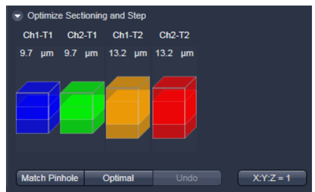
Fig. 79 Optimize Sectioning and Step: Optimal Interval is set starting with one Airy unit for all channels
