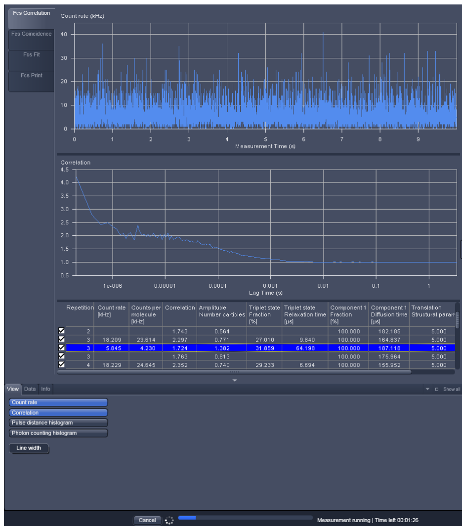
Fig. 117 FCS Correlation window during data acquisition
