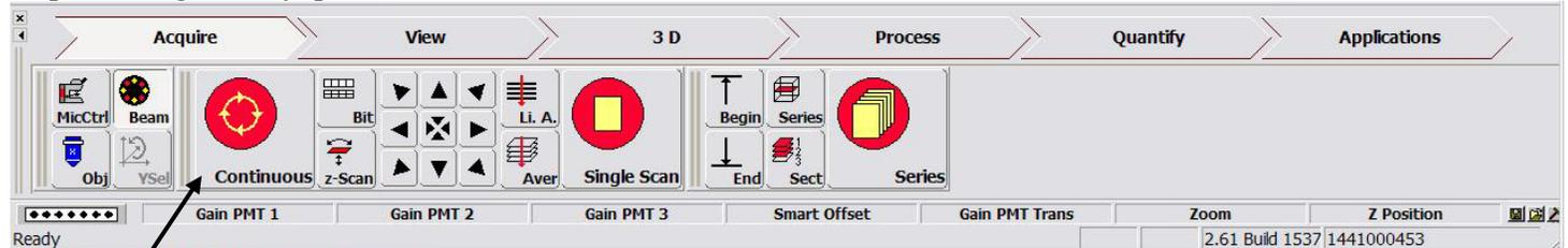
Press “**Continuous**” button to start scanning. An image or images, depending on the number of active detectors, will appear on the right monitor.
