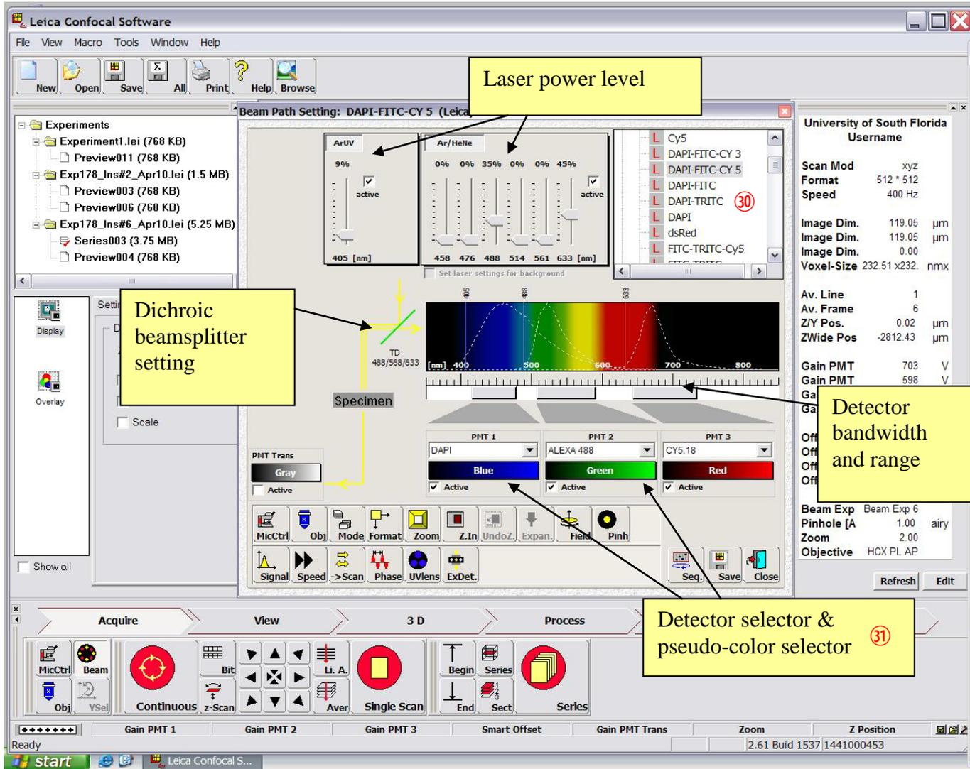
Click “**Beam**” button and select the appropriate detector setup for the fluorescent labels you used on your sample from the drop-down list <sup>30</sup>. This will set up the emission detector band-width, activate the proper detector (PMTs), dichroic beamsplitter, and excitation laser wavelength and power. You can adjust the range and position of detector bandwidth and the laser power level as necessary.
