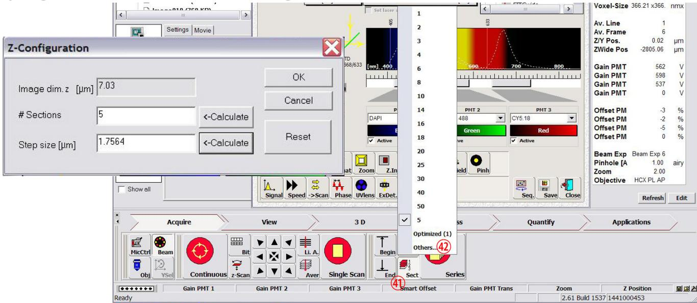
Click **Sect** button (41) to select the predetermined number of optical section, or to select **Others** (42)... It brings up a z-configuration window to determine the number of sections and spacing (step size) between sections. Press OK.
