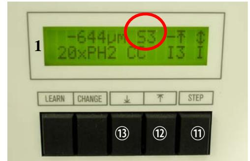
To focus, use **coarse movement button** (⑩ upper one for bring lens up to a safety distance, “0” position and lower one for lowering lens down) and **fine focus knob** (9) for focusing. The coarseness of focusing movement (“S0” (fine) to “S3” (coarse)) can be set by pressing “STEP” button ⑪.
