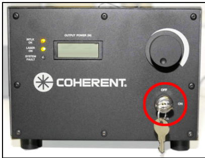
Figure 12: Key switch for the external UV laser
