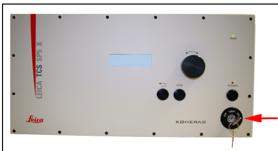
Figure 47: Detachable-key switch for the achromatic light laser
