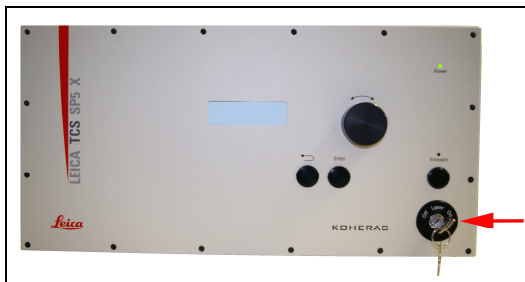
Figure 53: Detachable-key switch for the achromatic light laser
