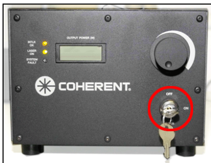
Figure 48: Key switch for the external UV laser
