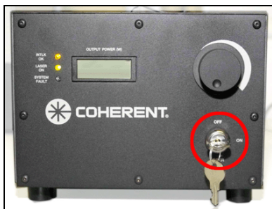
Figure 54: Key switch for the external UV laser
